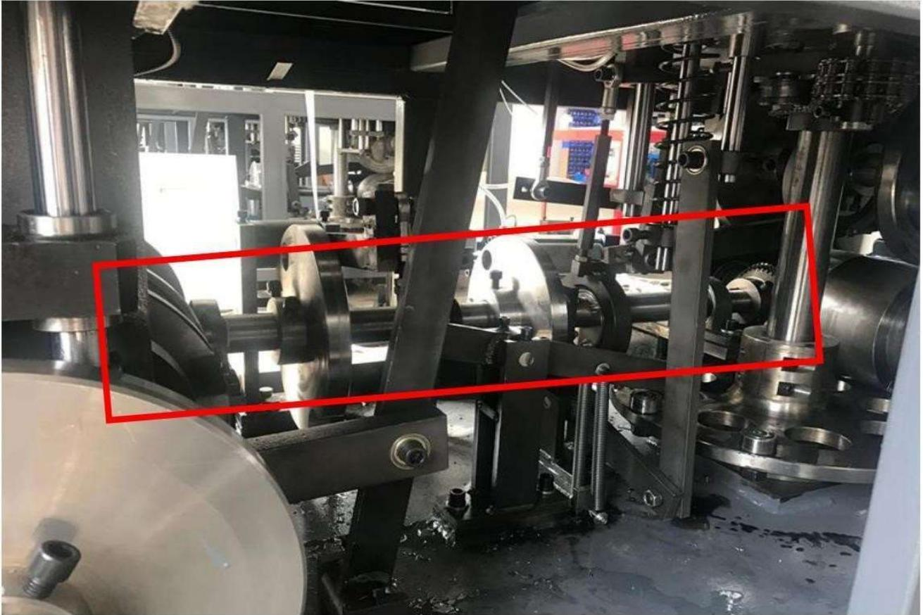
**Automatic Oil Lubrication System for oil lubrication machine moving**
