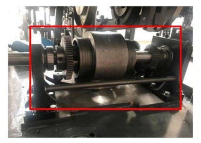
Main mechanism and moving parts are controlled by quality gears, which ismore efficient and more stronger than chain and axis.
