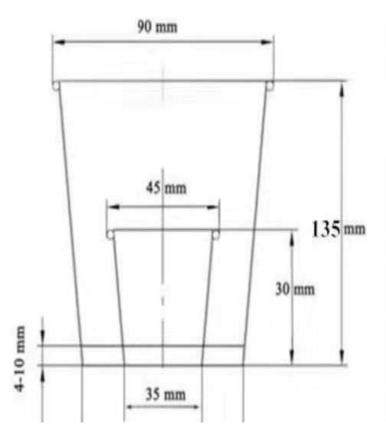
Cup Bottom diameter: Min 35mm ~ Max70mm
